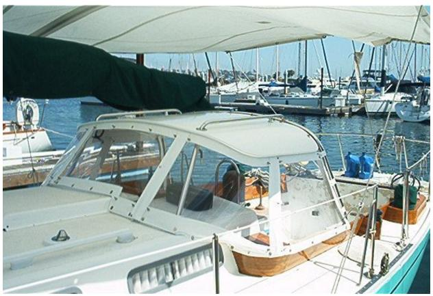
Notice the large flaps that completely cover the zippers. Keeping them out of them out of the sun was a key in the design. There was a plastic bolt rope sleeve attached to the inside of the dodger to capture the top of the material. Windows: Strattaglass, Material: Stamoid, Thread:Tenera
